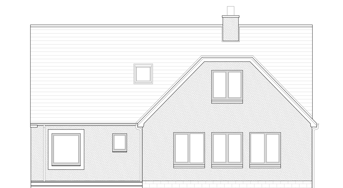
1:100 REAR ELEVATION AS EXISTING
